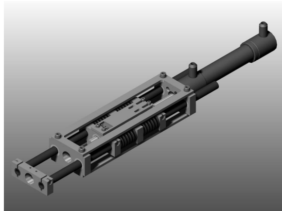
Fig. 1. Prototype Actuator CAD model. A 20MPa pressure source is connected to a MOOG series 30 flow control servo valve which has a bandwidth of about 200 Hz. The piston is coupled to the output through four die compression springs. The spring compression is measured with a linear potentiometer which implies force.
